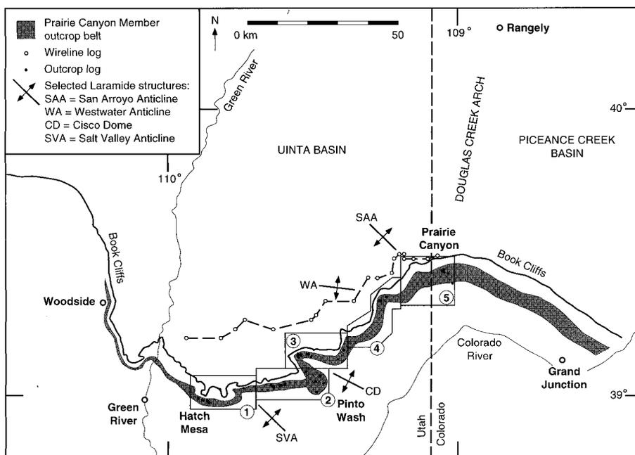
FIG. 1.—Map of the study area showing the Book Cliffs and the location of the Prairie Canyon Member outcrop belt south of the cliff line. The positions of detailed outcrop map and correlation panels 1–5 (Figs. 9–13) are referred to by circled numbers, and a subsurface correlation panel (Fig. 16) is shown as a dashed line north of the Book Cliffs. Key outcrop locations, discussed in the text, are shown in bold. Selected Laramide structures are also shown.
