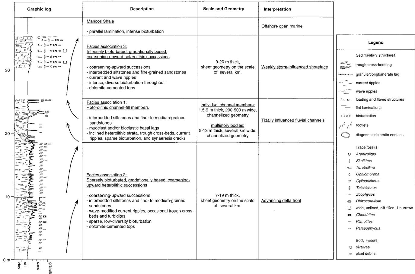
Fig. 4.—Schematic graphic log summarizing facies associations within the Prairie Canyon Member. Arrows to the right of the graphic log illustrate coarsening- and fining-upward trends. Note that most (approximately 60%) of the Prairie Canyon Member comprises open-marine Mancos Shale (Cole and Young 1991; Cole et al. 1997).
